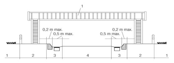
Sample cross-section of a street with a pedestrian bridge with installation-location groups
